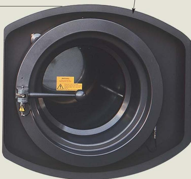
Extra-large loading door features computer-controlled PosiSeal™ lock which prevents door opening until final cycle is completed and all vapor has been removed from the system. Newly designed Cyclonic Airflo™ basket maximizes temperature-controlled air throughout the load for faster, more efficient drying and cool-down. It also features automatic back-plate washdown and residual lint removal. New rim design keeps buttons and other objects from getting lodged between the door and inside rim.
