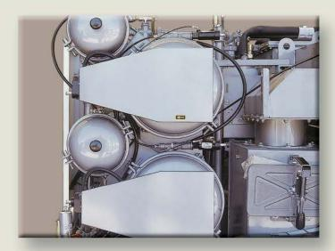
Multiple, independently functioning high-micron self-cleaning spin disc EcoFilters and large-capacity carbon cartridge filters are available on all Union 800 Series Systems to assure optimum filtration of both large and small particles for maximum solvent purity. Computer controls automatically pair filter operation for whites, darks or colors according to specific programs.
